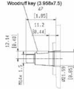
code 38 Max torque 250 Nm (2213 lbf in) European tapered 1:8
