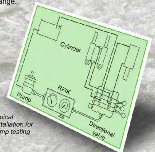
*Typical installation for pump testing*
