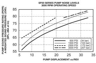
Pump acoustical data was determined in accordance with ANSI/B93.71M. Hydraulic fluid power-Pumps-Test code for the determination of airborne noise levels
