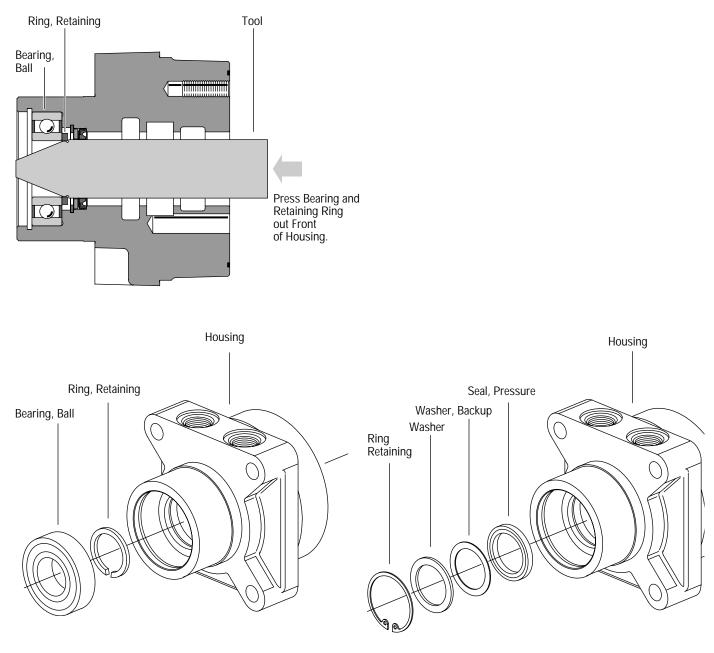
4 Remove bearing and retaining ring with special tool by inserting tool cone end first and driving these two parts out from back side of housing. Seal will be damaged when tool is inserted and must be replaced upon reassembly.
