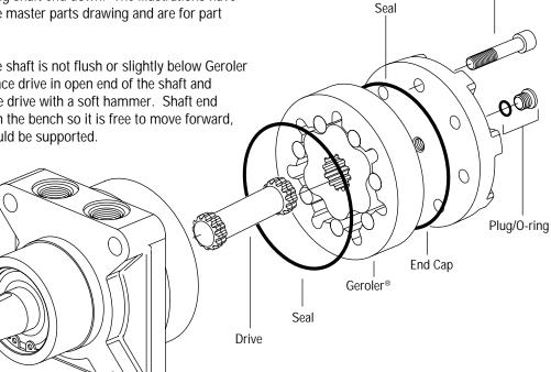
13 Install seal in seal groove of housing.
