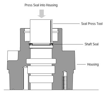
7 Position housing in the vertical position on a clean smooth surface, lubricate pressure seal with petroleum jelly and insert in housing, seal lip in the down position. Use seal press tool No. 600642 and press seal into position in housing.
