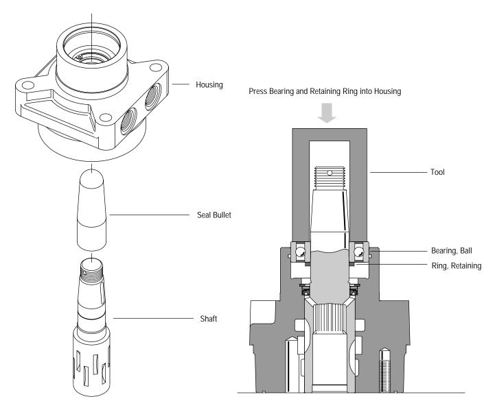
9 Place seal bullet over shaft. With bullet and shaft seal surface lubricated with petroleum jelly, place shaft on a clean smooth hard surface, output end of shaft up. Position housing over shaft and carefully lower housing over bullet and shaft.
