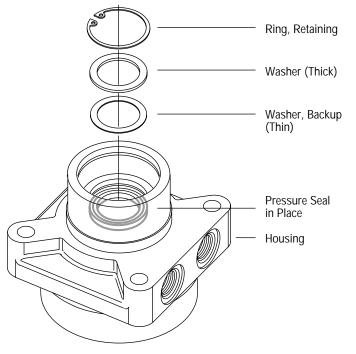
8 Place backup washer, washer, and retaining ring on top of pressure seal. Make sure retaining ring is fully engaged in groove in housing.
