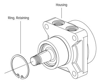
11 Install retaining ring, making sure retaining ring is fully engaged in ring groove in housing.
